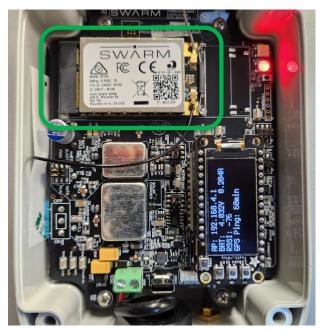
Swarm M138 Modem (PCIe Form Factor) Installed in Evaluation Kit
